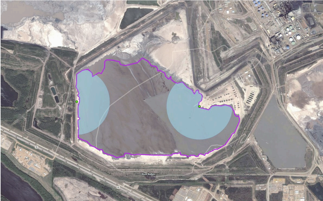
Figure 5.1. Example of survey station positioning at Suncor pond 2/3. Pond surface area is approximately 2.7 km 2 and circles illustrate 500m radius from survey station.
