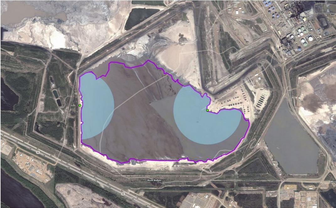
**Figure 1. Positioning of survey stations**
